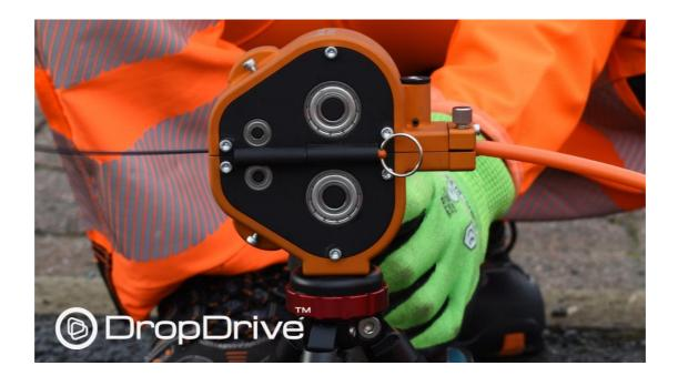
Emtelle's DropDrive™ achieves an industry-first pushing distances of 300m when combined with our REVOLink3 drop cable. Emtelle's cutting-edge drill-assisted pushing machine is designed to seamlessly enhance fibre optic pushing installations. Lowering overall deployment complexity, making installation accessible for all.
